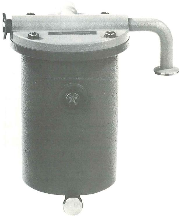
When the filter cartridge is clogged, the built-in safety valve opens and prevents the pressure during operation from becoming too high and damaging the filter and pump. The clogged filter element can be cleaned with appropriate solvents.
